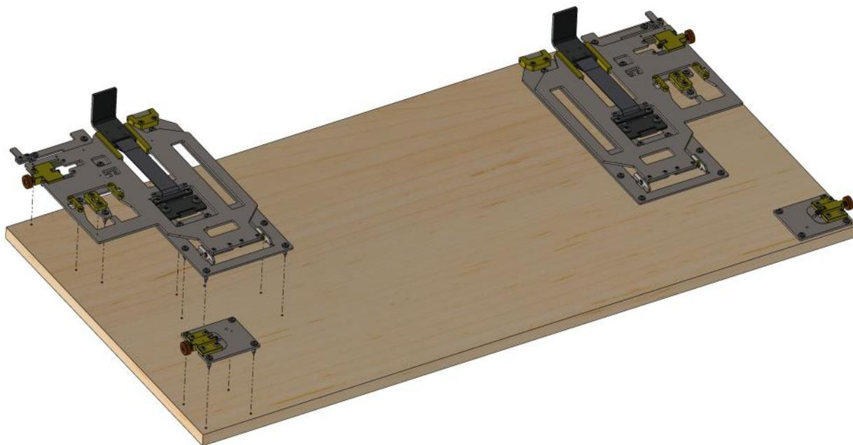
For **surface mounted panels**, provide the separately available 6 mm intermediate plate.
