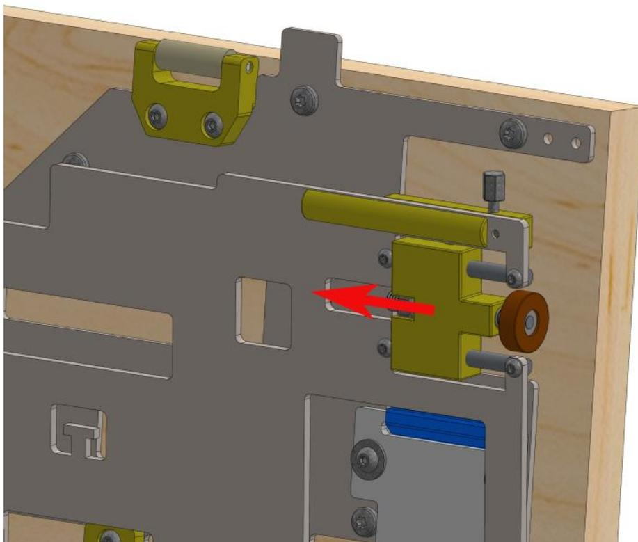
Insert the panel with the top wheels retracted into the corpus in such a way that the lower wheels enter the corresponding slot.
