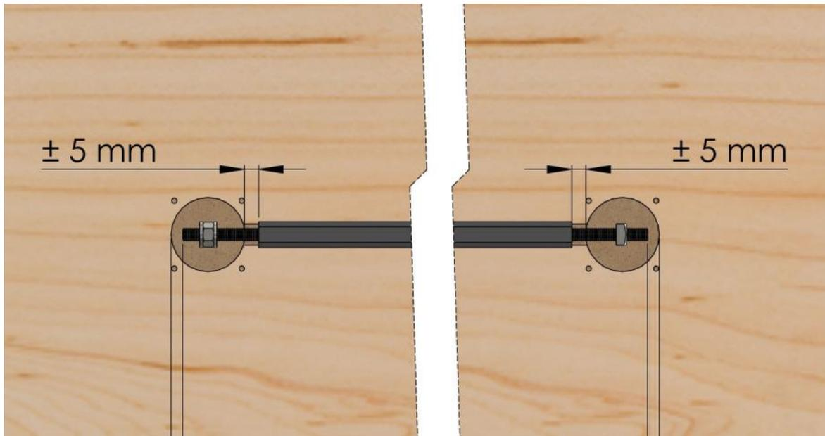
Place the retainers and threaded rod in their respective infreading (see drawings [www.Assunta.be](http://www.Assunta.be)).
