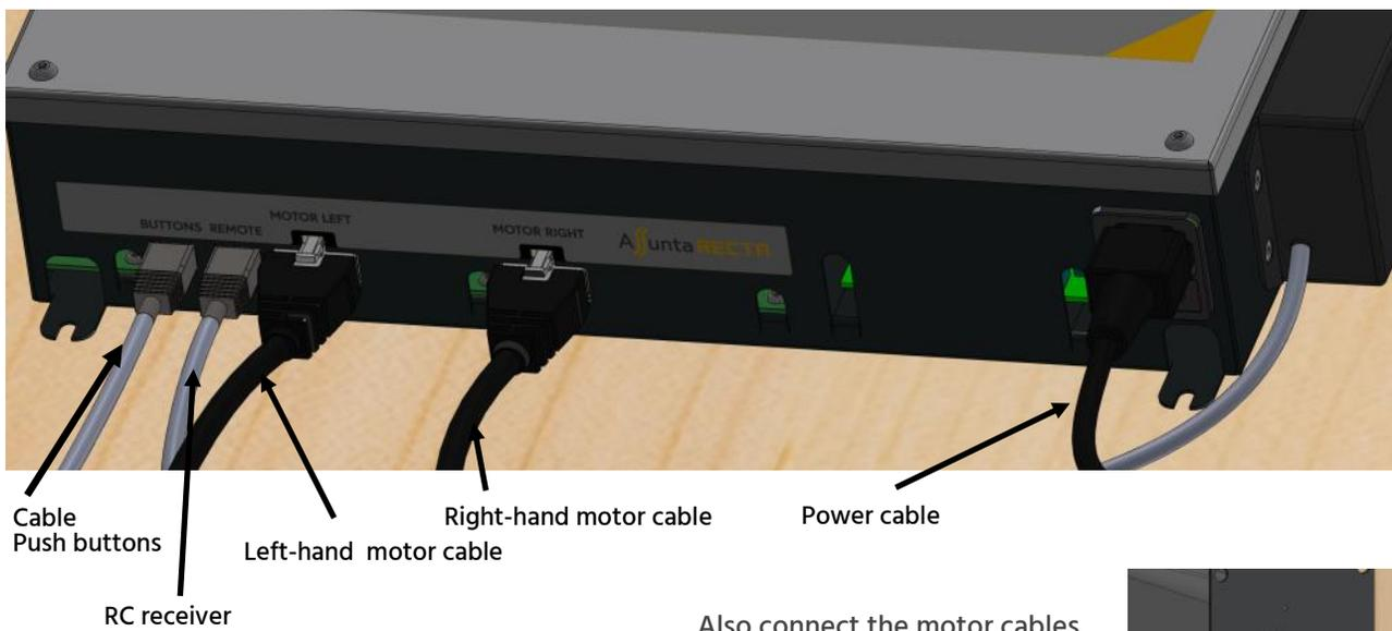
Also connect the motor cables on the motor side.
