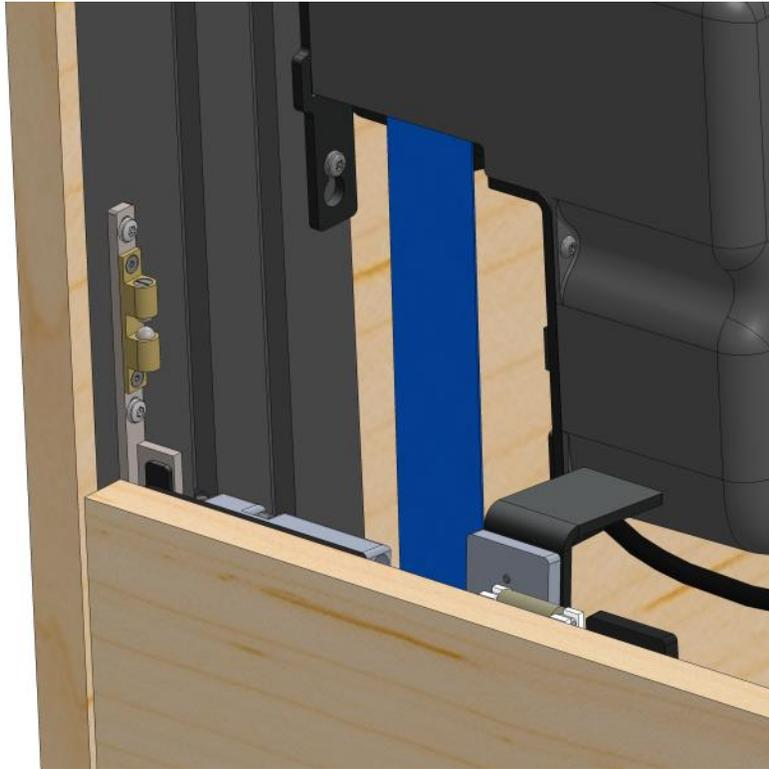
Place the fixed panel in the cabinet and unscrew the wheel of the hinge blocks into the groove provided for this purpose. Make sure the vertical clearance around the panel is evenly distributed.
