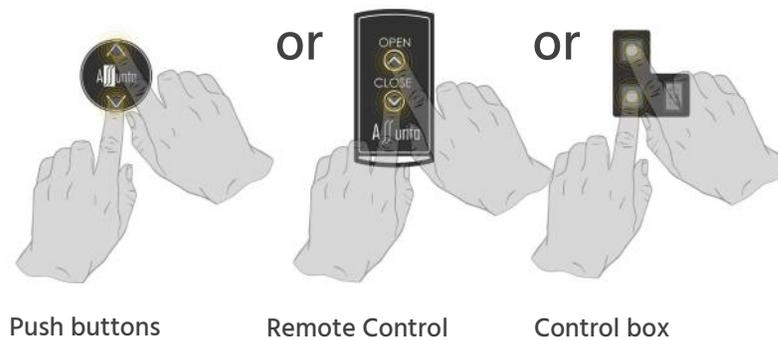
If the 'Adjusting' has gone well, place the system in 'RUN' mode by pressing and releasing the 2 control buttons simultaneously when 'R' appears (You will hear three beeps). The system will now first automatically perform an 'ADJUST' itself. After this adjust, the panel will come forward until against the next/fixed panel. When the panel is nice and straight, press the OPEN/UP button once and the panels will continue upwards. Once up, the system is ready for use.
