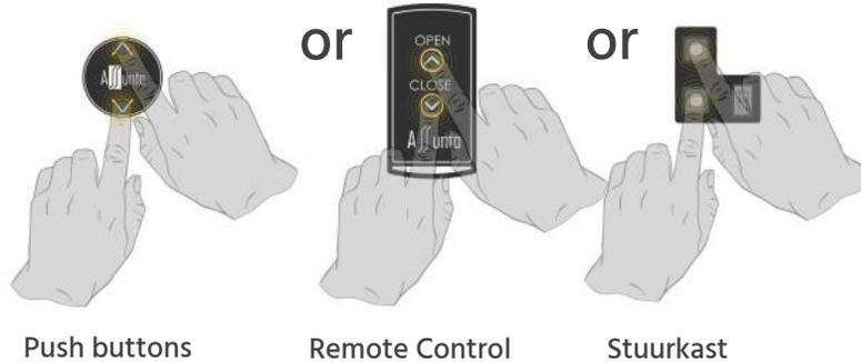
Place in the system in 'ADJUST' mode by pressing and releasing the 2 control buttons simultaneously when 'A' appears. (You will hear two beeps). The lower panel automatically positions itself on the bottom and the belts are tightened.
