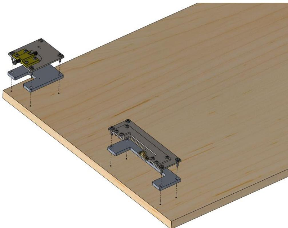
Screw the ball snappers to the side guides. Notice the adjustability in height and depth.
