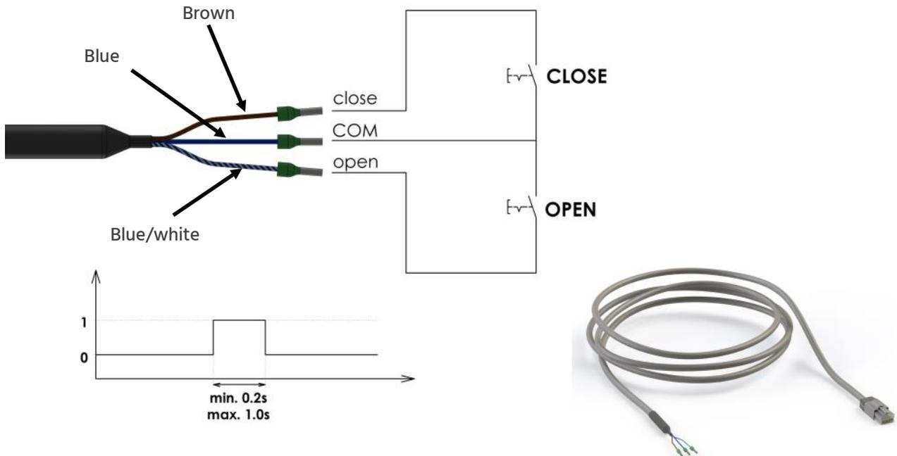
Proceed as follows to install any Assunta push buttons. Mill a recess according to the drawing below and glue the buttons in. Connect the RJ45 plug to the control cabinet. It must be plugged into the 'Buttons' socket.
