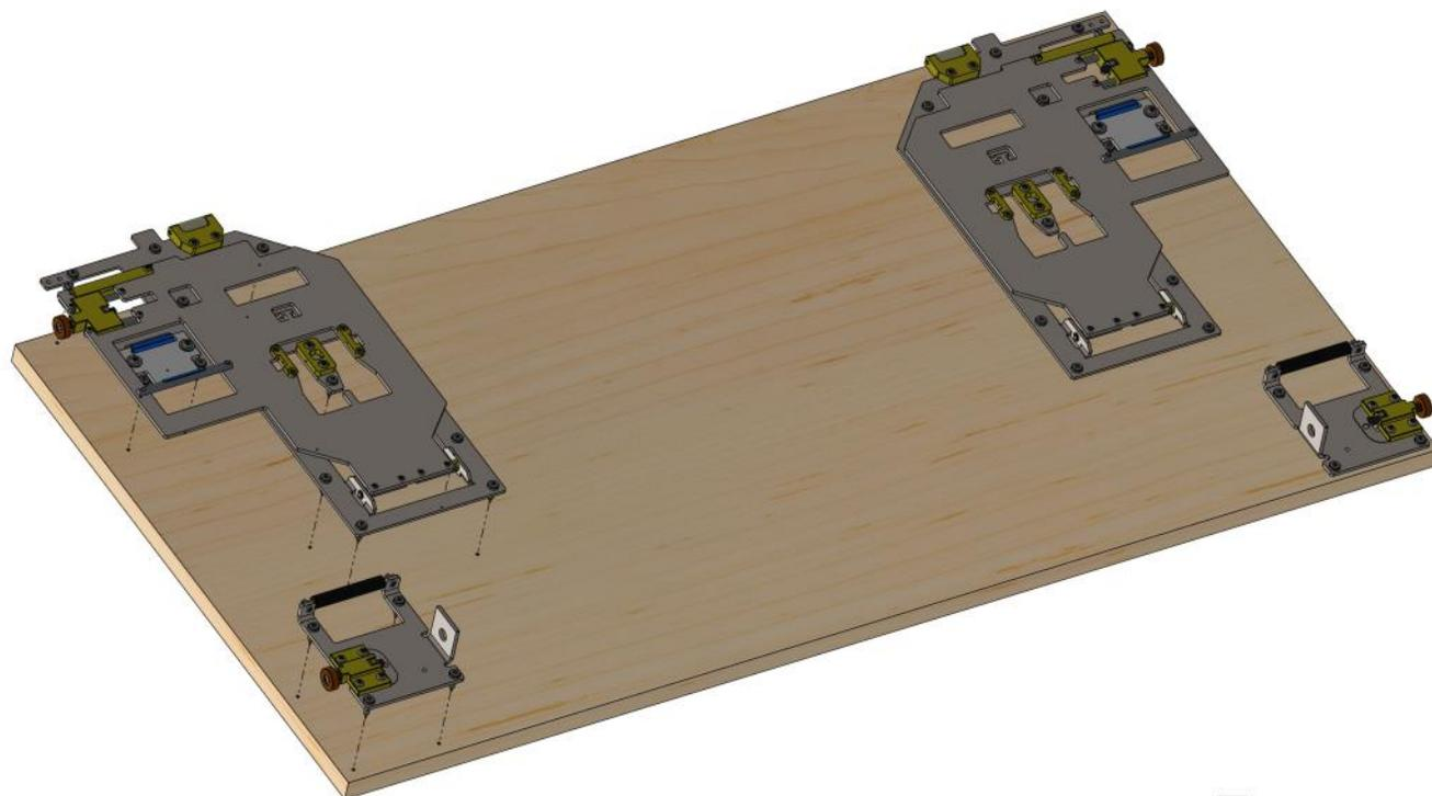
For **surface mounted panels**, provide the separately available 6 mm intermediate plate.
