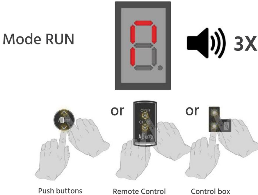
**AGAIN:** The 'measurement cycle' thus started when switching to mode RUN. RUN runs completely automatically except that you have to press the OPEN/UP button once when the lower panel straightens out. If you do not do this, the motors continue running and then return to bring the panel forward again. The panel will continue to oscillate in this way until you thus press the OPEN/UP button when the lower panel is straight.
