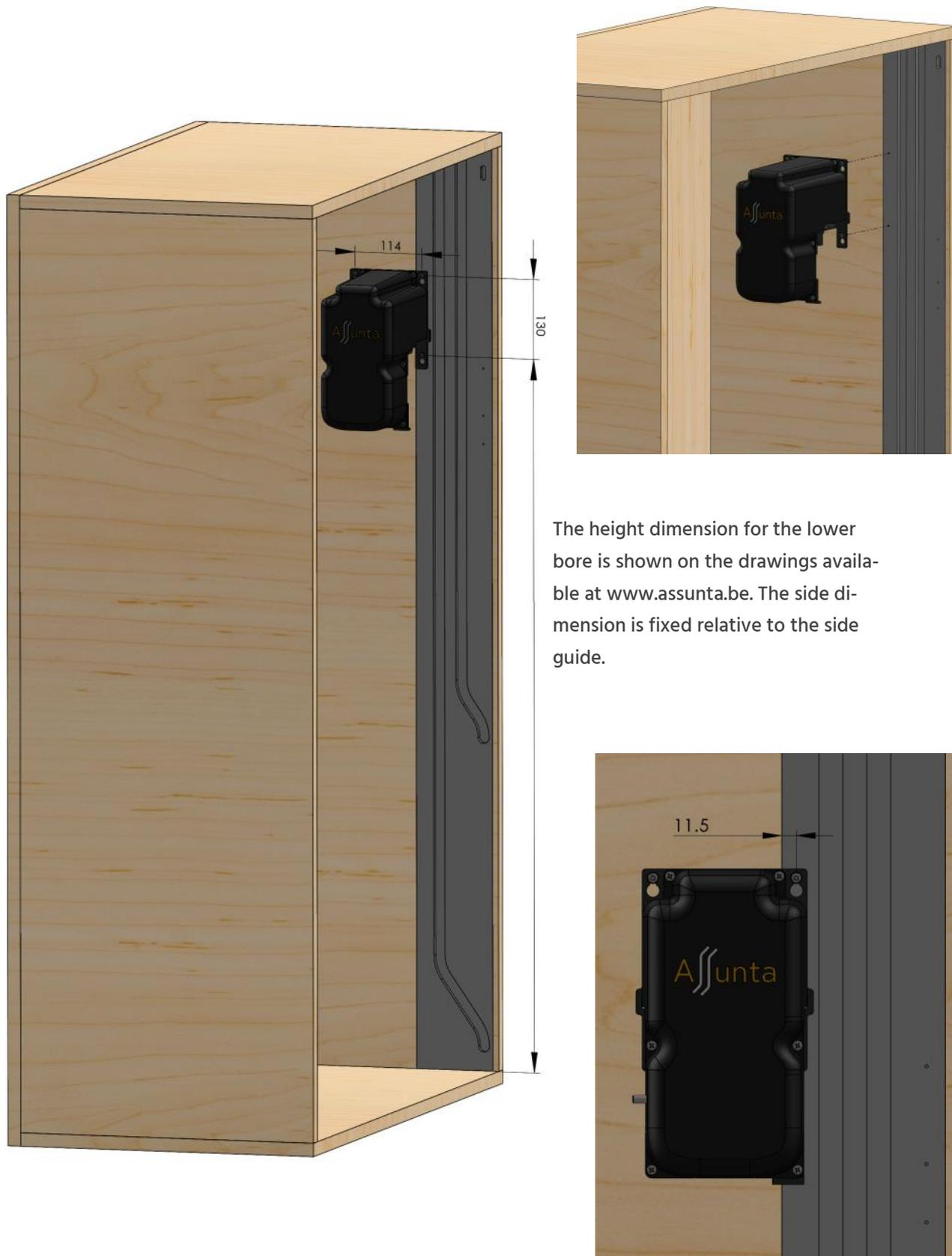
The height dimension for the lower bore is shown on the drawings available at [www.assunta.be](http://www.assunta.be). The side dimension is fixed relative to the side guide.
