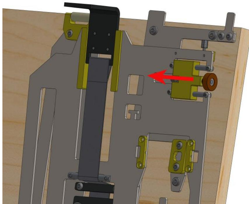
Insert the panel with the top wheels retracted into the corpus in such a way that the lower wheels enter the corresponding slot.
